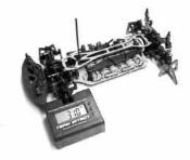
First, measure the left front weight. Write down this number on the worksheet for calculation.
