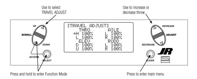
Press the *SELECT* key to select the desired channel then press the *INCREASE* or *DECREASE* key to select reverse or normal servo direction.
