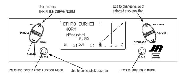
50%, 75% and high. Flight modes are located on the 3-position flight mode switch. The throttle curve is in the normal mode when the Flight Mode switch is in the rear position and the Throttle Hold switch is rearward.
