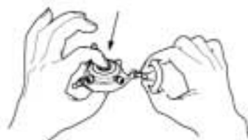
Swashplate Adjustment Test
