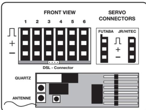
Disconnect the programming connector **within 10-20 sec** -> The receiver will switch to Hold mode. ( Fail safe positions are reset)
