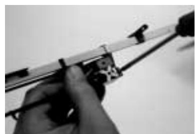
Carefully install the rubber tires onto the wheels and install the wheels on the main landing gear. Put on the stoppers. Insert the main landing gear into part B1.
