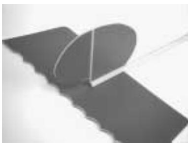
Cut the following plastic parts from the frame and insert them as follows: A8, B3, B4, B5, B1. Important : place the front wing holder B1 70 mm back from the rear edge of the motor.
