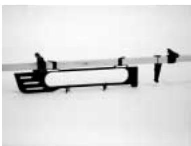
Glue the tail skid into the hole in the fuselage.
