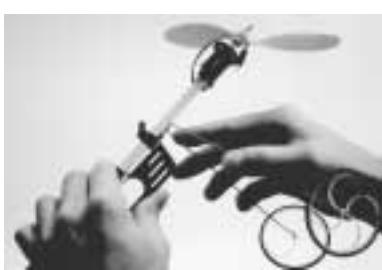
Insert the control horns to the slots on the stabilizer and the fin and fix them with the retainers. Insert the push rods into plastic support A8 and adjust the length. Bend the other end of the push rod and connect the control horns and servos.
