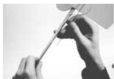
Place the receiver mount B6 on the CG point and glue it to the fuselage boom. Mount your receiver using the supplied double-sided tape. Fix the antenna on the fuselage boom with a tape. NEVER SHORTEN THE ANTENNA
