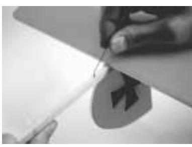
The centre of gravity is located 55 mm back from the leading edge of the wing. Use the battery to correct the CG position.
