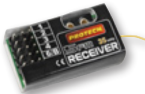
PRO.5-35 Micro RX FM - 35 MHz PRO.5-40 Micro RX FM - 40-41 MHz
