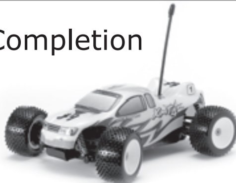
3. Put the body pin into the front body hole to fix the body to the chassis.
