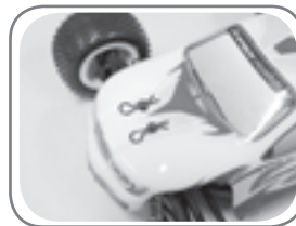
3. Put the body pin into the front body hole to fix the body to the chassis.
