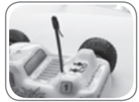
4. Put the body pin into the rear body hole to fix the body to the chassis.
