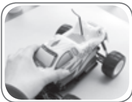
1. Put the body on the chassis.
