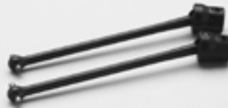
CVD center drive shaft (MIP style)
