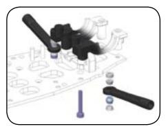
Adjust the rear toe-in linkage by changing the position of the thick spacer where the linkage connects to the rear block. This places the inner pivot point of the track-rod arm below, level with, or above the inner pivot point of the fixed rear lower arm.
