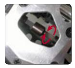
Stiffer rear anti-roll bar (linkage outer mounting hole):
