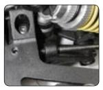
Upstops are used to prevent the front of the chassis from bottoming out on the pavement under braking.
