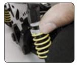
bar is tweaked. Loosen the screw on the left front anti-roll bar mount. Adjust the eccentric cam until both rear wheels lift from the ground at the same time. Tighten the screw to secure the adjusting cam.
