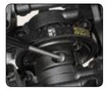
differential; loosen the adjustment screw to reduce the spin-resistance of the differential. The tighter the diff collar, the more the differential resists the difference in speed between the inner and outer wheel. Generally, the more grip a track has, the tighter the diff collar should be.
