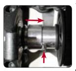
The 710 front one-way axle can be very quickly converted into a solid front axle by inserting two steel pins through the front axle and both drive adapters. An alu. bushing holds the pins in place.
