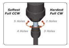
Serpent shocks can be assembled with nonadjustable or adjustable pistons. The nonadjustable pistons use a 1-piece piston with 2, 3, or 4 holes in it. The Serpent adjustable pistons use a unique 2-piece piston assembly that can be easily adjusted to align 2, 3, 4, or 5 holes.
