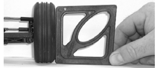
Testing camber with the camber gauge
