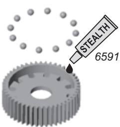
Fill ball holes with Stealth lube
