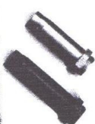
Fig. 13a Shock bodies come in different lengths and compressions.
