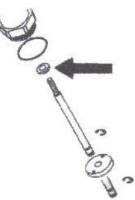
Fig. 20a Shock limiters will limit the amount of shock travel. This limiter will go inside the shock.
