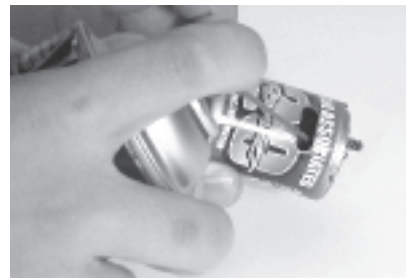
Spray the motor directly through the can onto the brushes and commutator.
