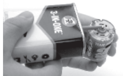
Apply a small amount of lightweight oil to each bushing for lubrication.
