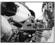
Locate the antenna tube in the plastic bag with the Operations guide. Remove the silver 5-40 setscrew from the radio tray with a 1/16" allen key (fig.2A). Thread the black antenna wire through the antenna tube (fig 2B). Push the antenna tube into the antenna mounting hole, then reinstall the 5-40 setscrew and attach the antenna cap.
