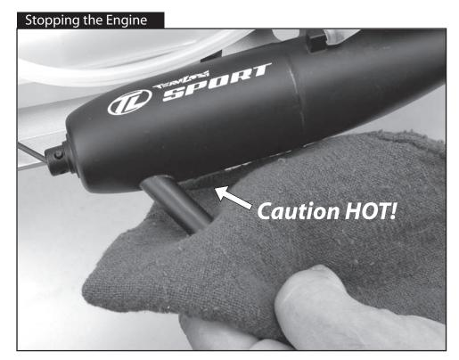
When you are done running your 8IGHT RTR, use the handle of a screw driver or a rag to cover the exhaust pipe exit. Be EXTREMELY careful not to burn your hand as this will be hot. Also, make sure turn the receiver switch off, then turn the transmitter switch off.
