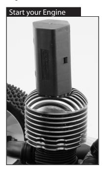
Attach the glow plug igniter to the glow plug. If you are using an aftermarket glow igniter with a meter make sure the needle is in the green or good condition. Holding the starter securely, press on the switch button and the engine should turn over and start.
