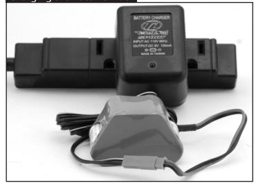
Plug the AC charger into the proper wall receptacle (110V). Plug the red male connector from the battery pack into the red female connector from the charger. When the battery is charging the red indicator light will be on. Charge for 8 to 12 hours depending on the level of charge remaining. Never charge for more than 12 hours. Never charge the battery wth the black battery connector connected to the black switch connector. Damage to your radio system may result.
