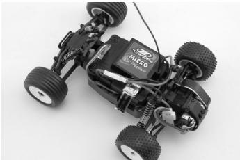
**5.** Plug in the battery lead into the speed controller lead and replace the body. Secure the body with the included body clips.
