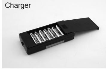
**2.** Remove the battery cover by sliding the cover in the direction noted on the cover. Install (8) AA alkaline batteries into the bottom of the charger. Pay close attention to the correct direction of the positive (+) and negative(-) ends as marked. Reinstall the battery cover.
