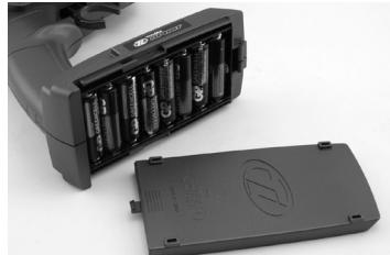
**4.** Remove the transmitter battery cover by sliding the cover in the direction noted on the cover. Install eight (8) AA batteries into the battery holder. Pay close attention to the correct direction of the positive (+) and negative (-) ends as marked. Once all 8 batteries have been installed, reinstall the battery cover.
