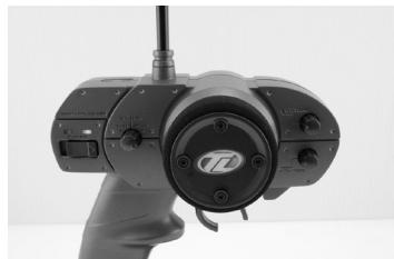
**6.** ALWAYS turn on the transmitter first by sliding the switch "ON". The small red and green lights above the switch should both light up. If not you need to check for low or incorrectly installed batteries.
