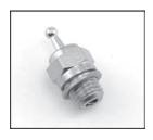
glow, remove the plug from the engine to check it in the same manner. A wet glow plug means there is excess fuel in the engine. To eliminate this, put a rag over the head and turn the engine over a few seconds with your "Spin-Start". Reinstall the glow plug making sure you have the brass gasket on it. The engine should now start.
