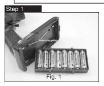
Remove the transmitter battery tray by sliding the bottom cover. Install eight (8) AA alkaline batteries into the battery holder. Pay close attention to the correct direction of the positive (+) and negative (-) ends as marked in the tray. Reinstall the battery tray using the molded pegs in the bottom as a guide for the correct location and replace the bottom cover.
