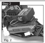
After removing the body, remove the small hatch pin just in front of the the receiver above the steering servo. Carefully swing the plate with the receiver/speed control upward and remove the battery box.
