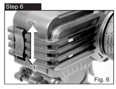
**Always** turn on the transmitter first by sliding the switch on the left side upward. The small red and green lights to the left of the steering wheel should both light up. If not you need to checkfor low or incorrectly installed batteries.
