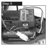
Intstall the battery box with the plug at the right front corner. Let the receiver/speed control plate drop over the batteries onto the mounting post and replace the hatch pin that secures it in place. Plug in the battery using the slots and bars molded into the plugs as a guide and your are ready to go!
