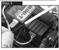
Insert the antenna wire through the antenna mount and into the antenna tube pushing it through until it comes out the other end. Push the antenna tube into the antenna mount.
