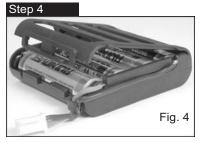
Remove the battery box top by lightly prying the bottom rail of either end of the retaining clip. Install four (4) AA alkaline batteries into the battery box, again paying close attention to the correct direction of the cells. Replace the cover and make sure the retaining clips snap over the railsat either end.
