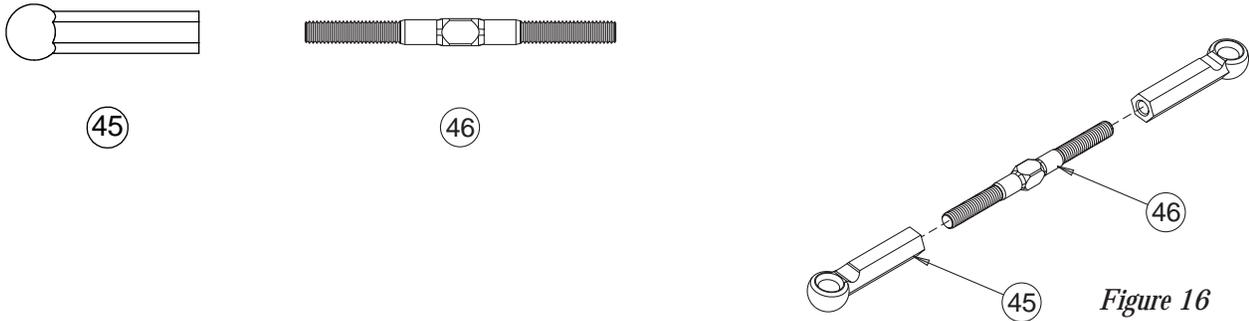
□ Step 25. Thread a plastic rod end (45) onto each end of a 1-1/2" turnbuckle (46). Tighten both rod ends (45) equally until the rod is the same length as the rod in Figure 16A. Make two of these tie-rod assemblies.
