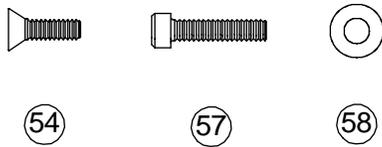
❑ Step 9. Place the rear shock tower (55) between the rear of the chassis (19) and the rear pivot block (49). The shock tower (55) should sit flat against the rear pivot plate (53). Place a #4 washer (58) over two 4-40 x 1/2" cap-head screws (57). Secure the shock tower (55) to the chassis (19) by threading the two 4-40 x 1/2" cap-head screws (57), with washers (58) attached, through the tower (55) and into the chassis (19).
