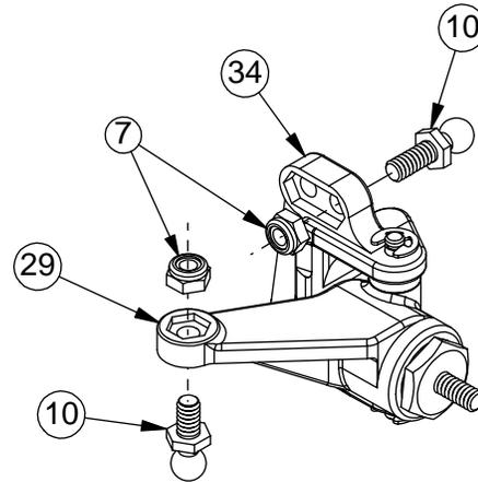
□ Step 13. Insert a 4-40 mini locknut (7) into the hex area in each spindle carrier (33), (34) as shown in Figure 11. Insert a 1/4" ball stud (10) into the outside hole (closest to the installed hinge pin) and tighten.
