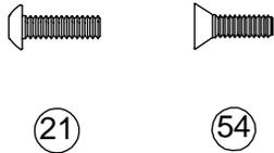
□ Step 1. Position the front bulkhead (20) on top of the front kickplate (14) and main chassis (19) as shown in Figure 7. Secure the front bulkhead (20) to the chassis (19) by threading two 4-40 x 3/8" button-head screws (21) through the hole in the top of the bulkhead (20) and into the chassis (19).
