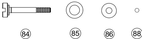
❑ Step 12. Locate the diff adjusting screw (84) and place the foam thrust bearing seal (85) over the shoulder of the screw (84) next to the head.
