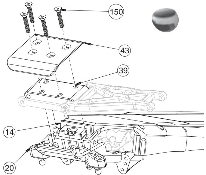
□ Step 20. Hold the chassis assembly upside down. Place the front pivot block (39) over the front edge of the front kick plate (14) as shown in Figure 13. The front edge of the front bulkhead (20) should be positioned between the front pivot block (39) and the hinge pin brace (42).
