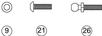
□ Step 4. Attach the front shock tower (24) to the front bulkhead (20) with four 4-40 x 3/8" button-head screws (21). The screws (21) thread into the top-most and bottom-most holes in the bulkhead (20). The center holes are not used.
