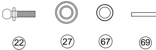
❑ Step 16. Thread a bluish ball stud (22) into the outer hole in the right rear hub (65), from the front (the side without the recessed area) as shown in Figure 22.
