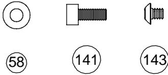
❑ Step 1. Attach the motor (*not included*) to the motor plate (96) using two 3mm x 8mm cap-head screws (141) and #4 washers (58). Do not tighten the screws yet.
