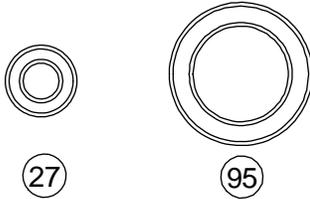
❑ Step 26. Insert a 3/16" x 3/8" sealed bearing (27) into the top bearing seat of the left gearbox half (94).
