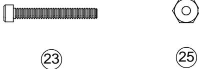
□ Step 3. Insert two 4-40 x 7/8" cap-head screws (23) – one on each side – through center holes in the top of the front shock tower (24). Secure the screws (23) to the shock tower (24) by threading a 4-40 nut (25) over each screw (23) and tightening.
