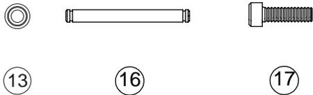
❑ Step 8. Insert a  $\frac{3}{32}$ " x  $\frac{3}{16}$ " ball bearing (13) into the two large, angled holes in the bottom of the front kickplate (14). Insert the other two bearings (13) into the two outer holes in the steering brace (15).
