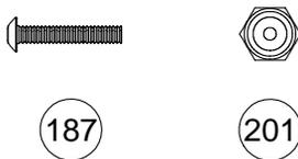
❑ Step 33. Attach the throttle linkage to the throttle servo horn by inserting a 2-56 x 1/2" button-head screw (187) through the over-ride slider (195) and into the inner hole in the longer arm of the throttle servo horn (190). Once the screw (187) is snug up against the over-ride slider (195), unscrew it one full turn to allow some movement between the arm (190) and the slider (195). Secure the screw (187) with a 2-56 locking nut (201).
