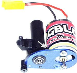
Now your motor is on the plate, make sure you have cut enough material at the arrow to allow motor movement
