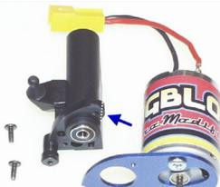
Removing a small part of plastic allows the use of small pinions. Use a file or a cutter. Install the rear block on the blue plates.
