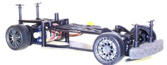
Now you are ready to go ! We suggest that you use a 12 teeth pinion to start. Make sure your speed control can manage the power of the Bigblock ! The use of team Orion 7.2 volts battery packs make it going even faster !
