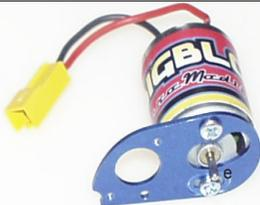
Install the motor on the blue plate with the (e) screw on the top and the (f) screw on the bottom.
