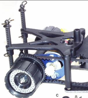
Use the (d) screws and insert the (c) spacers to fix the rear body holder on the chassis.
