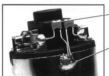
.1uf capacitors (2): Solder as shown from motor wires to motor body.
