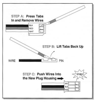
IMPORTANT: Wiring the plug incorrectly may damage the speed control or radio receiver, and will void the warranty.
