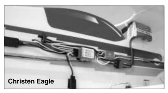
32.Connect the servo wires to receivers and speed controller as shown. You will need one servo extension to connect aileron servo. Use Velcro to secure battery as photo shown. Secure the RX and ESC with the furnished Double-Sided tape. Organize the wires and fix them on fuselage with tape if necessary.
