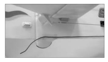
33. Route the antenna wire to the tail and tape it on fuselage.
