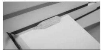
8. Epoxy the tail in place. You may use the rest triangle balsa wood and epoxy it at the bottom of horizontal tail.
