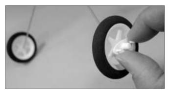
15.Install wheels by threading the wheel pant retainer in proper position.
