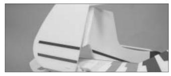
11.Use the furnished tape to tape the Rudder in place. Tape the left side first then the right side.
