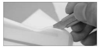
Locate the tail skid, next use hobby knife to cut a slot at the bottom of fuselage tail. Then insert the tail skid in place.
