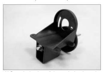
27.Press the bearings all the way in then insert the Spur Gear Drive Shaft. Snap on the E clip. Try pull the drive shaft and make sure E clip is well positioned and drive shaft will not come off.
