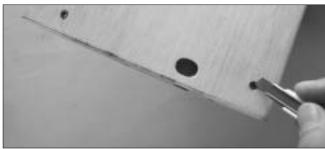
2. Cut away the covering at servo hatch, the hole near the wing root where extension wire to go through and mounting holes.
