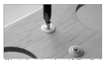
32.Locate the plastic washer and 3x20mm Wood Screw then secure the tail on the T-tail mount. Make sure the horizontal tail is perpendicular to the vertical tail and has same angle to the main wing if you see from the nose.
