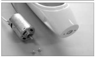
37.Locate the motor, and 3x8mm countersunk screws. Secure the motor in the fuselage.
