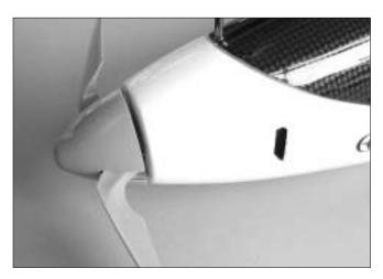
39.Make sure there is about 2~3mm(5/64"~1/8") gap between spinner backplate and fuselage.
