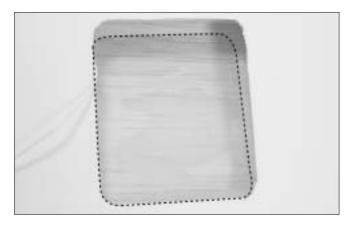
4. Sand the glue area of the plastic square piece (servo bed) then CA it on the wing planking.
