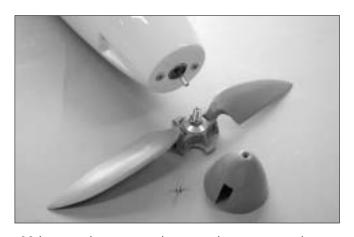
38.Locate the prop, spinner and screws as shown. Assemble the folding prop first. Make sure the two blades move freely. Insert the drive nut to the backplate then the drive shaft. The hole of drive nut is tapered to accommodate the drive shaft. Secure the whole set onto motor shaft with the nut. Do not over-tighten the nut as it might break the aluminum drive shaft but make sure it will not spin out when it in high rotation.
