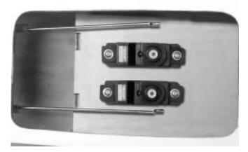
40. What we used here are mini servos. You may use standard servo but need to enlarge the servo tray. The upper one is elevator servo and lower one is rudder servo.
