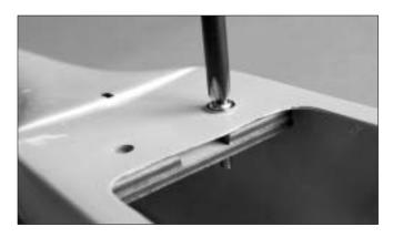
23.Install the blind nut in place. Secure the wing bolt all the way in with the blind nut underneath the wing mount.
