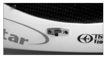
45.Use switch plate as a template, drill holes then install the switch as shown.
