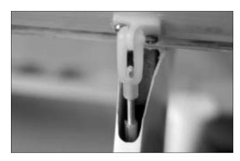
34. Snap the clevis onto the control horn as shown. It may need to file the T-Tail portion to make sure the movement is free.
