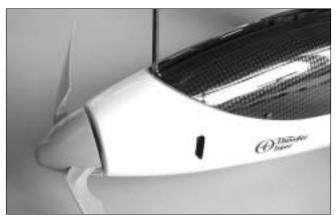
47. With the canopy in place on the fuselage, drill 5 holes with 1/16" (1.5mm) bit. One in the front of canopy, two at both sides of the canopy. Next secure the canopy with 2x5mm wood screws.
