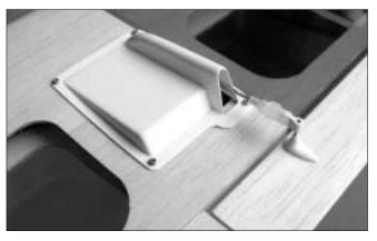
14.Next secure the Hatch Cover in place with furnished 2x5 mm wood screws. Snap on the clevis on control horn. Thread a small piece of silicone tube and slide it on the clevis to prevent it from loose.
