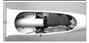
42.Refer to the manual of Electronic Speed Control Unit (ESC-50 Shown P/N:ACE8014), link to motor, battery and receiver. You may wrap the receiver with sponge or thin foam pad. It will protect the receiver and reduce the vibration from motor.
