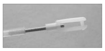
33.Locate the short/ long threaded end, clevis and plastic tube. Thread the long threaded end to plastic tube first abut 1/4" (6mm) in length then insert the plastic tube through the guide tube from the bulkhead end. Get the plastic tube at the rear of T-Tail mount then install the short threaded end and clevis.
