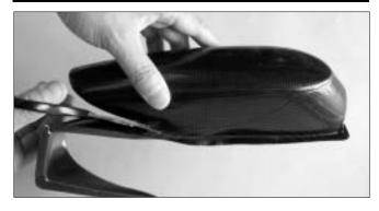
46.Locate the canopy. Cut 1/16"(1.5mm) outside the molded line with curved scissors. Trial fit and trim it until it fits on the fuselage.
