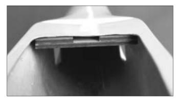
17.Glue the front and rear wing mount in place either by thick instant glue or epoxy. The wing mounts are flush with the opening of fuselage.
