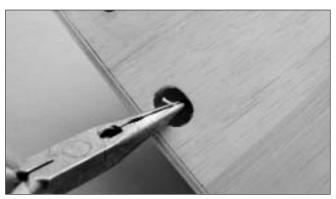
8. Pull the string out from the hole slowly, using needle-nose pliers or tweezers.
