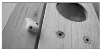
30.Drill 2mm holes and install the control horn on the tail, note it has to be in line with the tail mounting holes and the control horn is even with the elevator leading edge.
