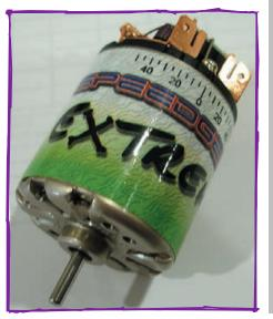
Brushless motors go bad when the rotor loses its magnetic strength due to the demagnetizing effects of the stator while the motor is under power. When this happens the motor will lose bottom end, run hotter and eventually burn up the stator windings.
