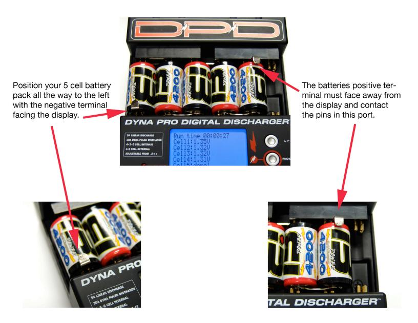
Your DPD Phase II Discharger will now discharge and condition 5 cell matched battery packs. The discharging process is exactly the same as when processing 4 and 6 cell battery packs. The only difference is placement of the battery pack in the DPD discharger. Your battery pack has to be loaded using the five ports on the left. The negative battery terminal must face the display and the positive terminal must face up. Just follow the pictures above and you will have no problems.
