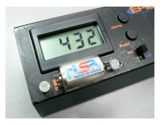
To test D3/IRRA slot car motors place motor between the cradles up against unit. Rotate motor 180 degrees and than press hold button.
