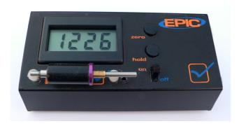
In the default setting, the checker is in the **real time strength mode**, indicated by a "C" after you turn on the unit. Put the rotor in the cradles and slowly rotate the rotor forward and backward through 180 degrees. The LCD will display the varying magnetic strength from the highest to lowest point as the field changes from positive to negative. Be sure to go past the highest point of magnetic field on both the positive and negative sides to get the most accurate reading.
