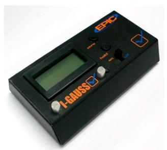
By pressing the ZERO button with no magnet nearby or sitting on the cradles the calibration is completed when "000" shows up on the meter. The checker is then ready to be used.
