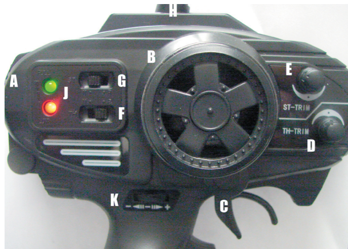
A - ON/OFF Switch: Controls power to the transmitter. B - Steering Wheel: Steers the vehicle left and right.
